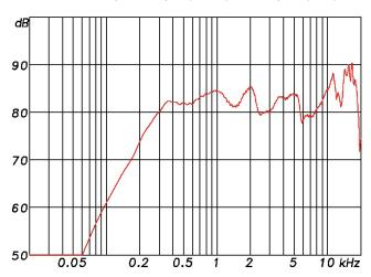
RL 110 AX-MP3 max. SPL @ 3% and 10% distortion threshold 30 W max. Power
