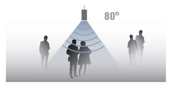
Minimum lateral sound radiation and a short distance allows focused acoustic irradiation to the visitors.
