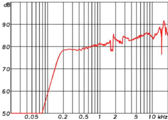
S 2 A max. SPL @ 3% and 10% distortion threshold 20 W max. Power
