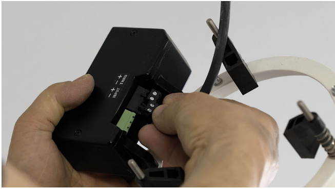
Insert terminal at input of crossover.
