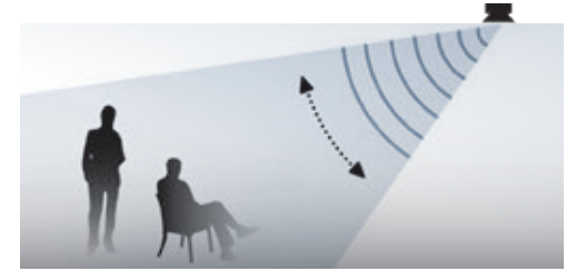
DE Plan 800 AIArray, in-ceiling installation with adjustable directivity
