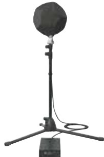
Miniature dodecahedron speaker for room acoustic measurements
