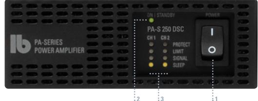
1 Power switch The amplifier switches on with a delay of approx. 3 seconds.
