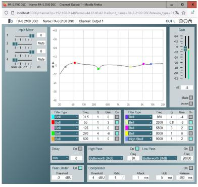
Browser-based app for configuring and controlling our amplifiers and active speakers with digital signal processors (DSPs). One or more devices can be connected via Ethernet and configured using the **LB AUDIO CONTROL app**.
